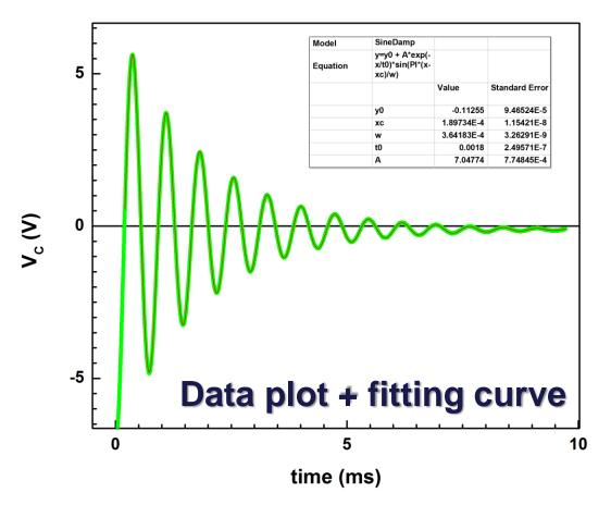
$$q(t) = Ae^{-at}sin(\omega t + \varphi)$$
