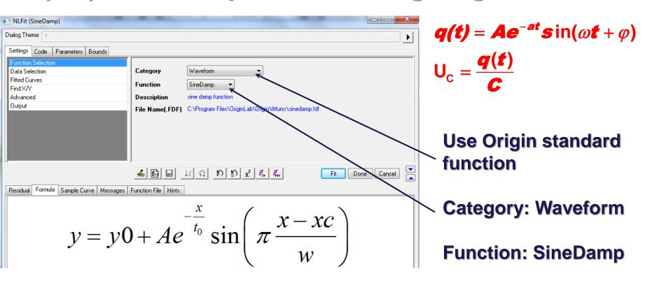
Fitting function; y0,A,t<sub>0</sub> xc, w – fitting parameters
