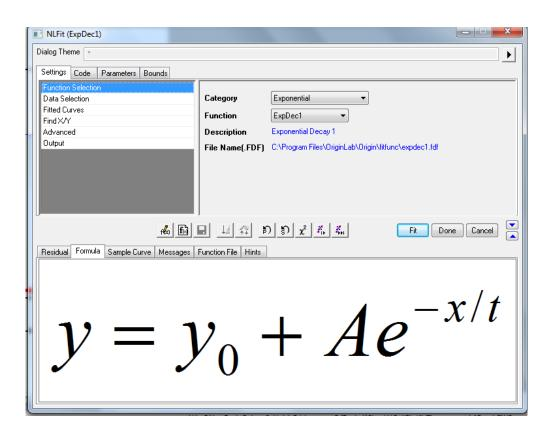
Fitting the "envelope data" to exponential decay function
